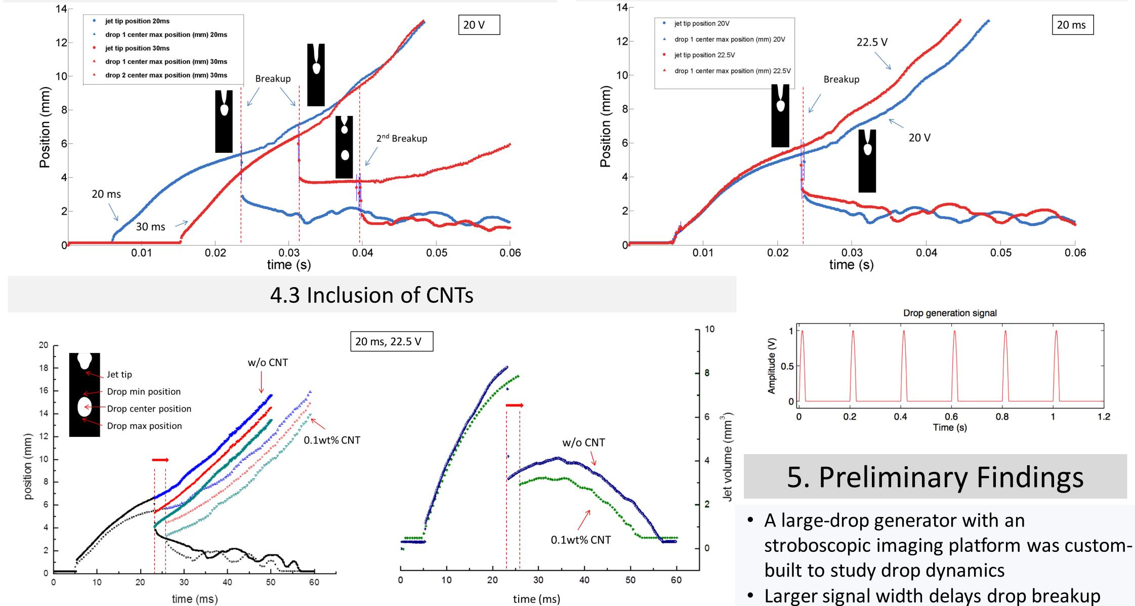
Drop generation signal: sinusoidal signal with a pulse width and voltage indicated in the figure. Ten images were taken at the same delay time every 0.1 ms for glycerol/water mixture and every 0.5 ms for CNT suspensions.
